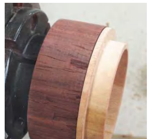
STEP 27. Mount the rosewood lid into the chuck and hollow the inside to accept the apple insert. Once you have a really good fit, glue the liner in but you need to make sure the glue is dry before moving on to the next stage
